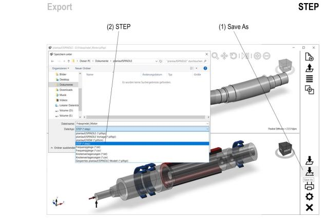
Export the geometry as a STEP file (button "Save As" and file type "STEP"). The file includes the spindle geometry, the additional masses and the bearings.
