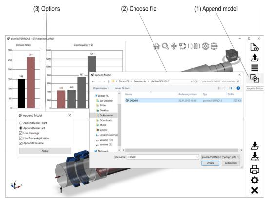
Existing models can be appended to the current one with the "Append Model" command. Choose the file and select the option to append the model to the **left or right**. Select the option to import the bearings if appropriate. Appending tools to spindles usually requires to use the forces' location at the TCP. You can also combine the filename of the current model and the appended one.
