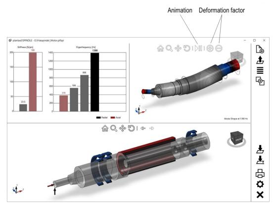
Static deformations and mode shapes are shown in the animation area. Use the symbols to ncrease/decrease the deformation factor and to start/stop the animation.
