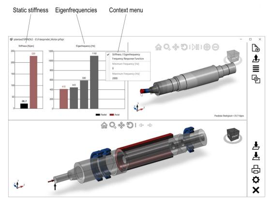
The results are shown in the top half of the window. If the option "Stiffness / Eigenfrequency" is chosen the results are displayed as bar diagrams on the left. Click on a bar to visualize the deformation or the mode shape on the right. **Black (red)** bars represent radial (axial) deformations or mode shapes. There are six eigenfrequencies that can be shown. If needed the frequency range can be changed in the context menu of the diagram.
