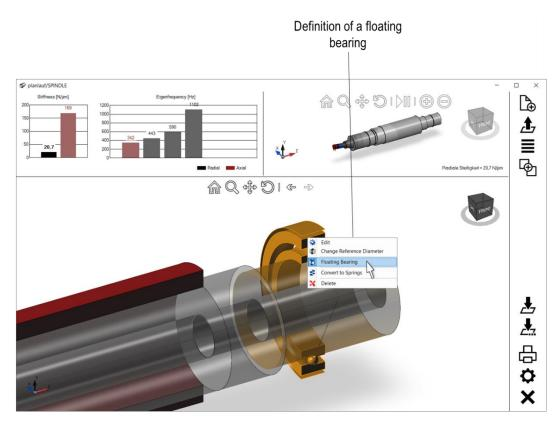
Some bearings are used as floating bearings and don't contribute to the axial stiffness of the bearing set. Select the "Floating Bearing" option in the context menu "Bearings" to set the axial stiffness to zero. Floating bearings are marked with an additional ring.
