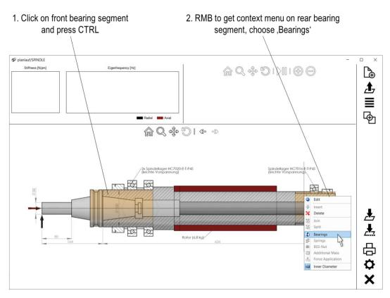
Spindle bearings are usually used in sets, so the front and the rear seat are not on the same segment. In addition, the diameter of the front and rear seat can be different. Define a set of spindle bearings on two different segments (one segment is also possible) with the following steps:
