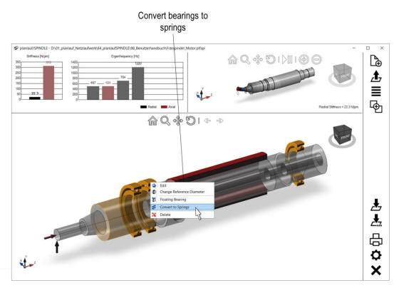
Springs with translational and rotational stiffness and damping values can also be defined (context menu "Outer diameter" > "Springs"). Additionally, bearings or bearing sets can be converted to springs (context menu "Bearings" > "Convert to Springs") or be taken from a database. Move the springs with the same mouse dragging operations as the bearings.
