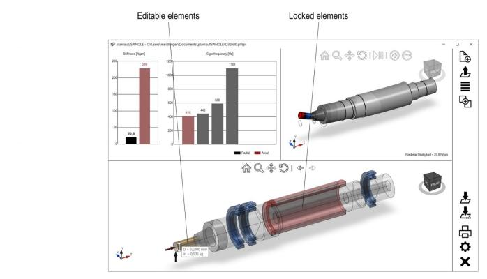
The combined model contains the editable elements of the tool and the locked elements of the spindle. Locked elements are shown more transparently and are also not accessible through the context menus or the tables.
