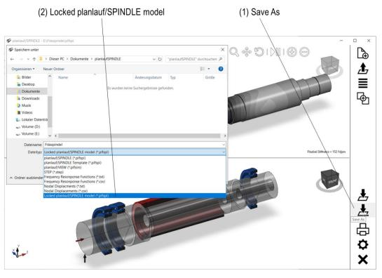
planlauf/SPINDLE models can be saved in a locked state where no changes are possible anymore. This format is useful if a spindle manufacturer wants to provide a simulation model to one of its customers. The customer can then calculate the eigenfrequencies for different tools. Click on the "Save As" button and choose the file type "Locked planlauf/SPINDLE model" to save the file with the extension \*.plfspl.
