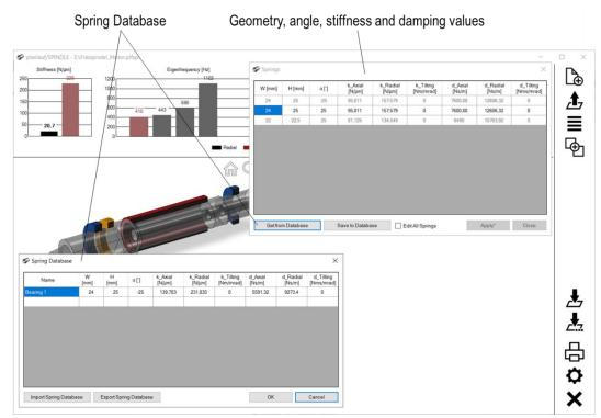
**Remark:** The **angle** (negative: to the left, positive: to the right) considers the stabilizing effect of X arranged bearings.
