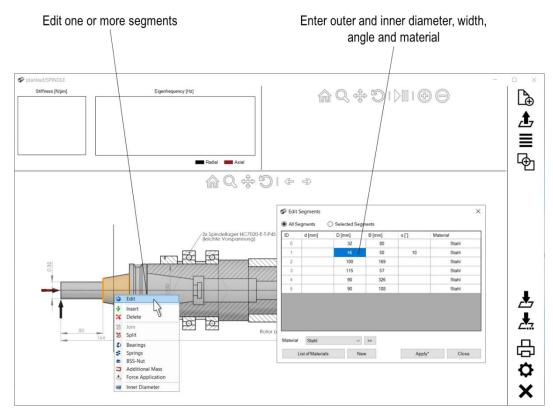
Apart from the dragging operations, the geometry can also be modified in the segment list. **Doubleclicking** on a segment/selection or the "Edit" command in the context menu "Outer diameter" will show the list.
