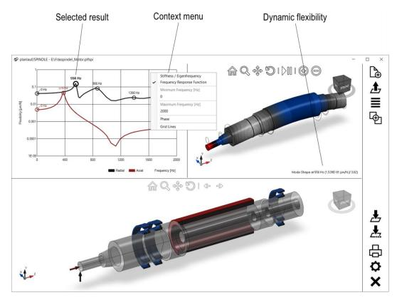
The results are shown in the top half of the window. If the option "Frequency Response Function" is chosen the radial FRF (black) and the axial FRF (red) are displayed. Click on the small circles in the diagram to display the deformation or mode shape on the right.
